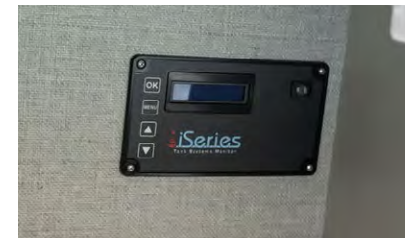
Figure 4-3. Tank Level Monitor
