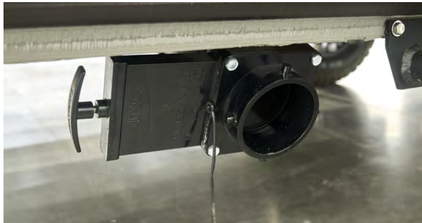
Figure 4-5. Grey Water Tank Drain
