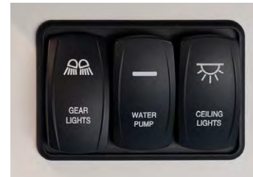
Figure 5-6. Switch Control Panel
