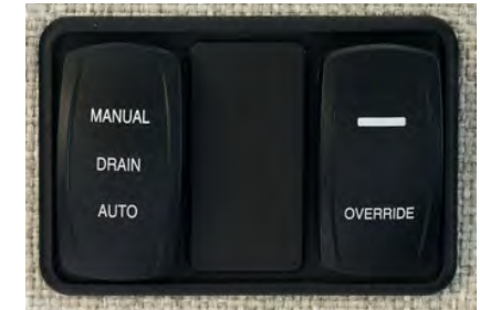
Figure 4-6. Shower Drain Switches
