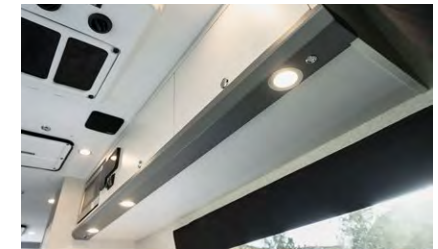
Figure 5-8. Reading and Galley Lights
