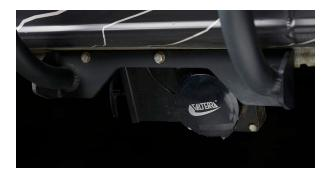
Figure 4-5. Grey Water Tank Drain
