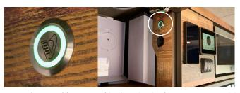
Figure 2-1. ON/OFF Pushbutton and its location in the upper Connectivity Cabinet
