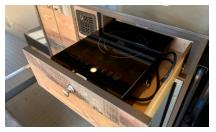
Figure 5-21. Portable induction stove storage drawer
