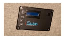
Figure 4-3. Tank Level Monitor
