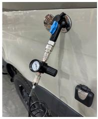
Figure 4-14. Quick connect stud and quick connect coupler
