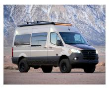
Figure 6-3. Exterior lighting — Light Bar with Amber Setting, Side Lights, and Fog Lights
