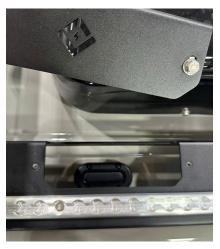
A cable port has been added to the ceiling panel in the Connectivity Cabinet for ease of installation of cell boosters or satellite antennas like Starlink. To open the cover pull down on the cover, the SCANSTRUT pass-thru is directly above this cable port.
