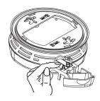
Figure 1-2. Battery Compartment
