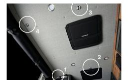
Figure 4-11. Shower curtain's connection points and recommended order of installation
